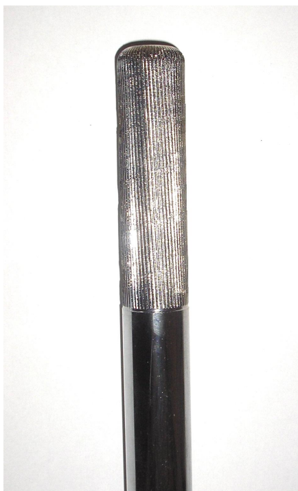
Foto from the steering column with the section with the knurling for the steering wheel hub (knurling according to DIN 82 - RAA1).
